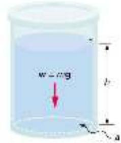
$$P = \rho \cdot g \cdot h \quad \left\{ \begin{array}{l} \text{Or} \\ \rightarrow \rho = \frac{P}{g \cdot h} \\ \rightarrow h = \frac{P}{\rho \cdot g} \end{array} \right. \quad \left\{ \begin{array}{l} p = \text{pressure at point A in (pa)} \\ \rho = \text{density of liquid in (kg/m}^3\text{)} \\ g = \text{gravity in (N/ kg)} \\ h = \text{height of liquid above point A in (m)} \end{array} \right.$$
